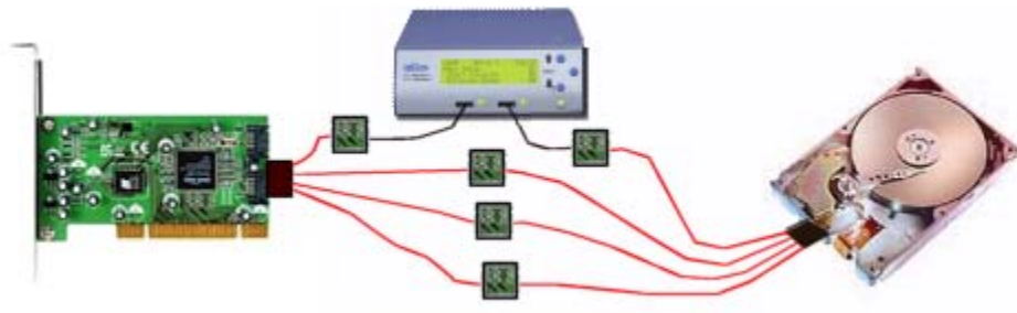
Figure 18 Multiple Connections Using "Octopus" Cables
